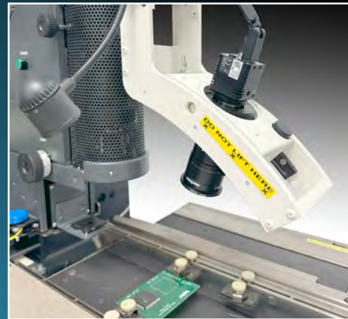
Precision Vision Alignment - Inspection-Quality Microscope or High Definition Camera
